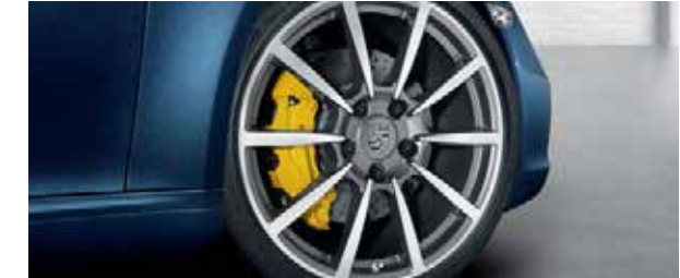
Porsche Ceramic Composite Brake (PCCB)
